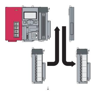
2. Replace the A/D converter module.
