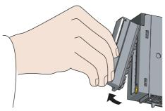
2. Use the terminal block fixing holes as a fulcrum and remove the terminal block.
