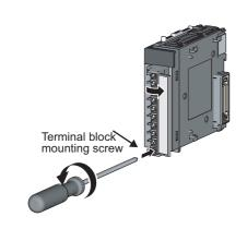
Open the terminal cover and loosen the terminal block mounting screw.
