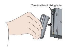
Fully insert the projections on the top of the terminal block into the terminal block fixing holes and press the terminal block until it snaps into place.
