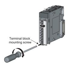
2. Open the terminal cover and tighten the terminal block mounting screw.
